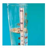
2. Post-production analysis is mandatory if either ethanol or an isopropanol solution is used. Use the alcoholmeter to control the alcohol concentration of the final use solution. The accepted limits should be fixed to ± 5% of the target concentration (75%–85% for ethanol).
